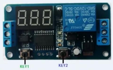
☆KEY1: Bit selection, to choose hundreds place, decade and the unit. Long pressing the KEY1, can close or open the Digital tube.
